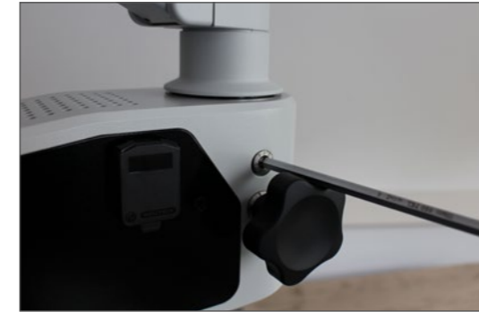
1. Loosen the hexagon socket wrench screw. The needed wrench is enclosed.
