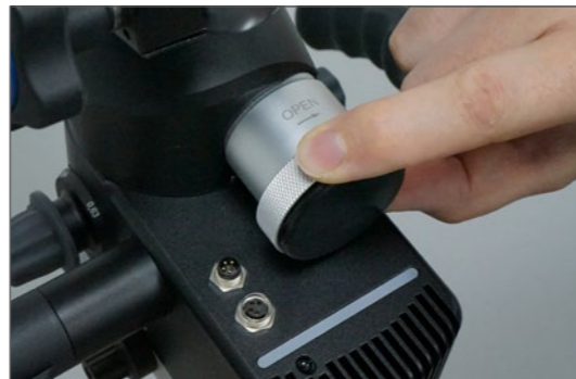
4. Remove dust guard from optical connector.
