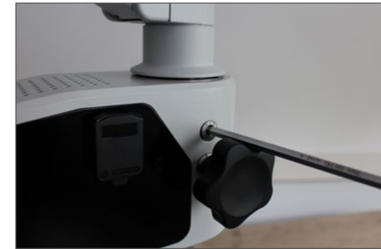
3. Tighten the hexagon socket screw.
