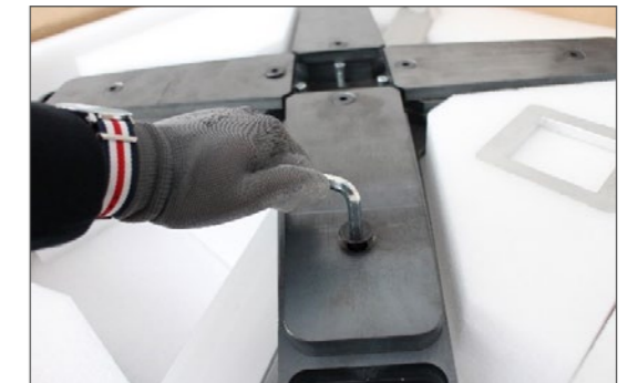
2. Remove the balance weights by loosening the screws with an 8 mm Allen key. The screws are secured at the bottom with M12 nuts (wrench size 19 mm).
