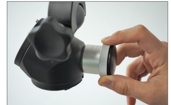
2. Remove dust guard from optical connector.
