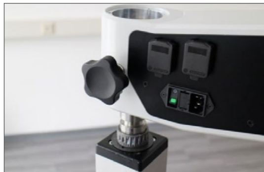
5. Attach suspension arm to guide bearing.
