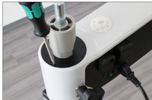
6. Assemble mount (take care of angle position).
