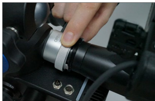
5. Fit adapter in optical connector and save with ring.
