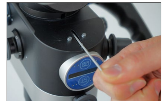
6. Assemble lighting unit to ergo optic (2 mm Allen wrench).
