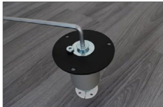
4. Components assembled (take care of countersunk position).
