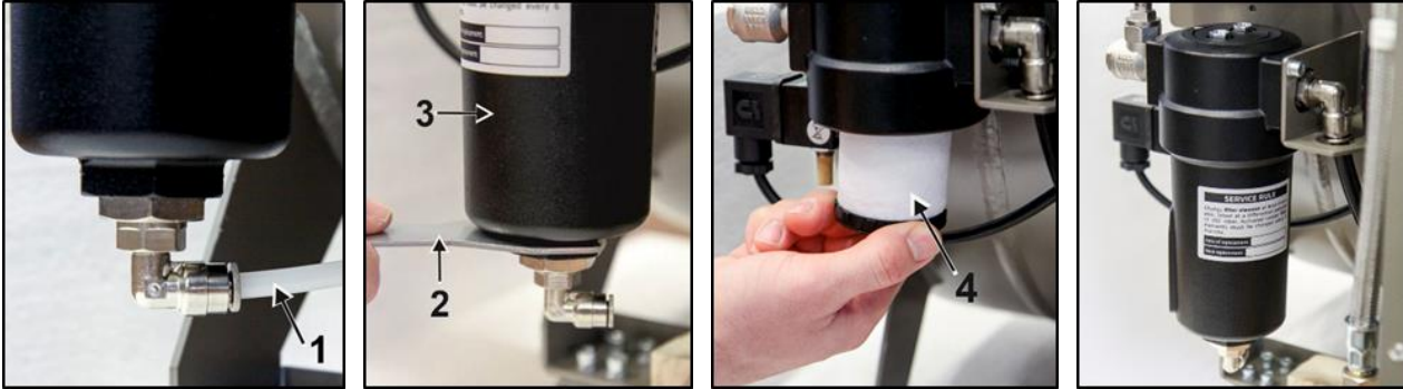
Fig. 19: Filter element replacement
