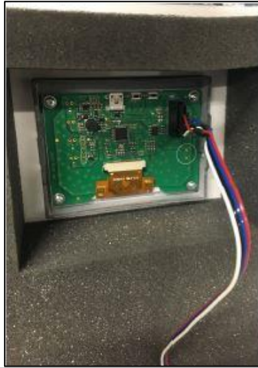
Fig. 17: Connecting the display connector
