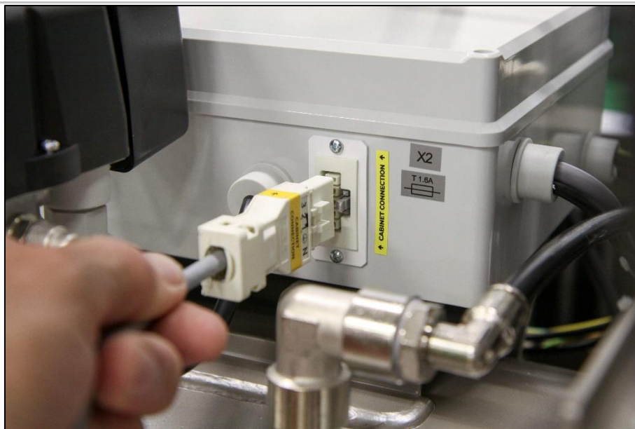
Fig. 13: Connect the cabinet to the compressor
